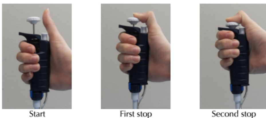
Figure E3. Relative locations of first and second stops when depressing the plunger of a micropipette. Image source: Boston College Investigations in Molecular Cell Biology lab manual.
